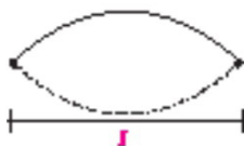
Fig. 4-23: Fundamental mode of vibrating string
